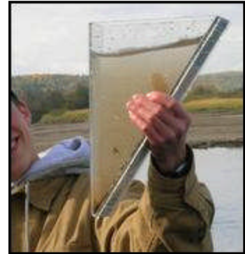
Turbidity wedge, used to evaluate how 'muddy' the water is.
